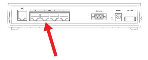
If you add devices connected through a hub or switch, connect the hub or switch to an Ethernet port on the Netopia 3366-ENT.
